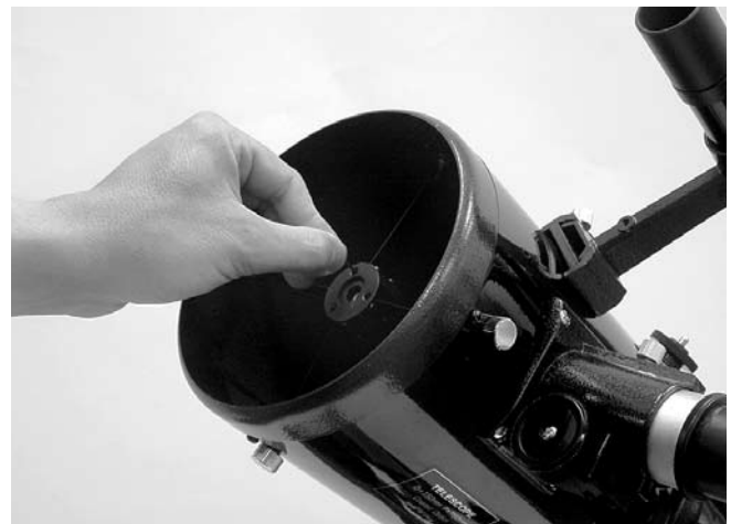
Figure 12: Adjust the tilt of the secondary mirror by loosening or tightening the three alignment set screws with a 2mm Allen wrench.
